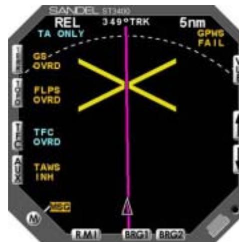
**TAWS FAIL:** (Shown below in TOPO mode). FLTA and PDA alerts and display are disabled due to lack of required data.
