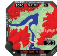
FAA released draft guidance outlining the technical requirements for a widely expected mandate that will require the installation of terrain awareness and warning systems (TAWWS) on all helicopter EMS (HEMS) aircraft.
