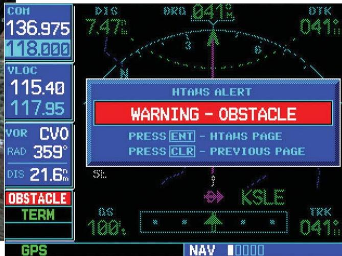
GNS 430/540W navigators with Garmin HTAWS includes operating modes for Normal and RP (reduced protection) modes.
