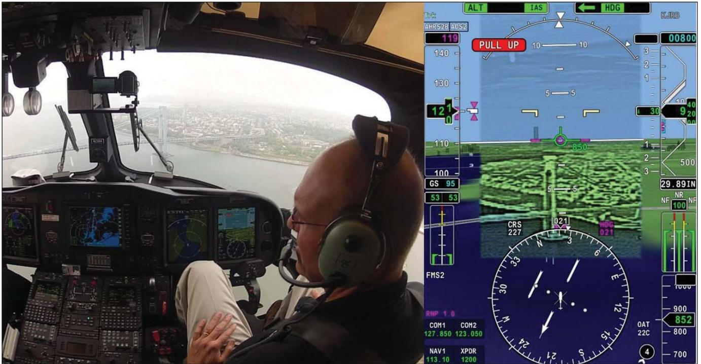
Honeywell's Marc Lajeunesse puts the new SV-HELO TAWS through the paces over New York City. This is the helicopter industry's 1st real Combined Vision System (CVS) bringing HTAWS into the Primary Flight Display (PFD) and merging wire and obstacle data with enhanced vision.
