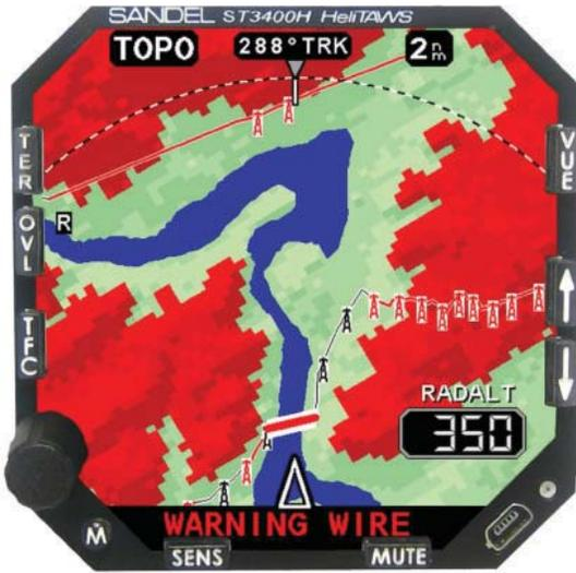
Sandel's ST3400H HeliTAWS was designed as a nuisance-free alerting system to warn helicopter operators flying very close to the ground, power lines and wires.
