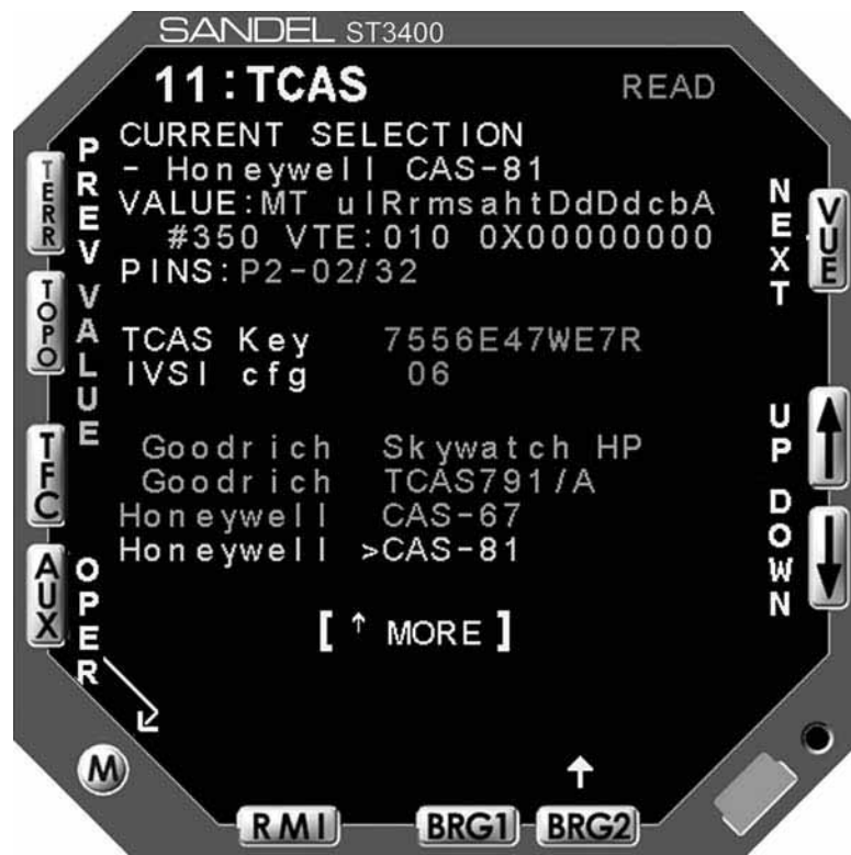
Figure 6-9: TCAS Select Maintenance Page (typical)
