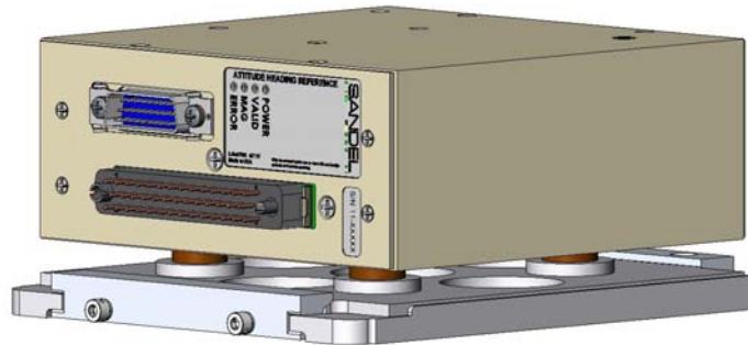
Figure 3-3: SG102-0xx w/MOD1, -1xx, -2xx, -3xx installed in Mounting Base Assembly
