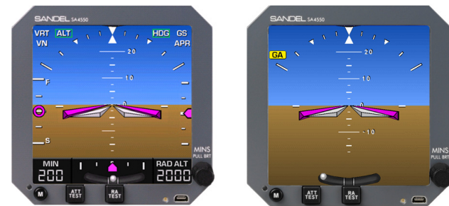
Figure 2-6 SA4550 Primary Attitude Display
