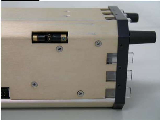
Fig. 1: Place SN3308 unit upside down on a grounded bench area.
